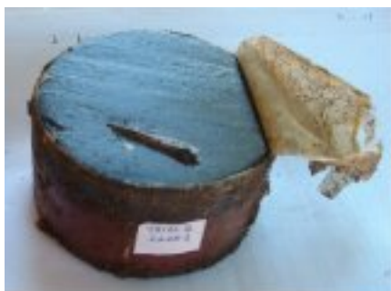
The damaged GYATA surrogate is shown on the left (with the latex witness plate peeled back).
